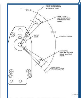
gure 6-2. Mechanical End Stop and Switch Actuation Point Adjustments
